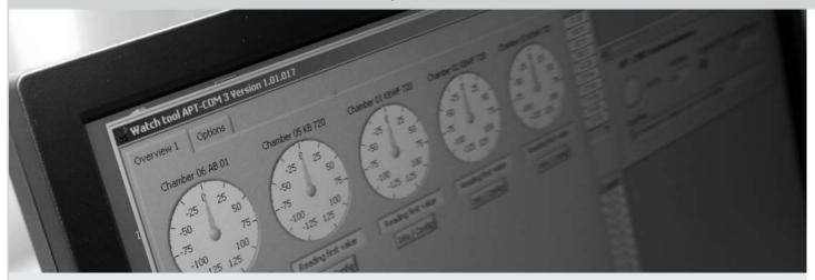
Software package APT-COM™ 3 DataControlSystem for Windows to network up to 30 units or controllers with the communication interface RS 232 or RS 422 for remote control, programming and data recording.
