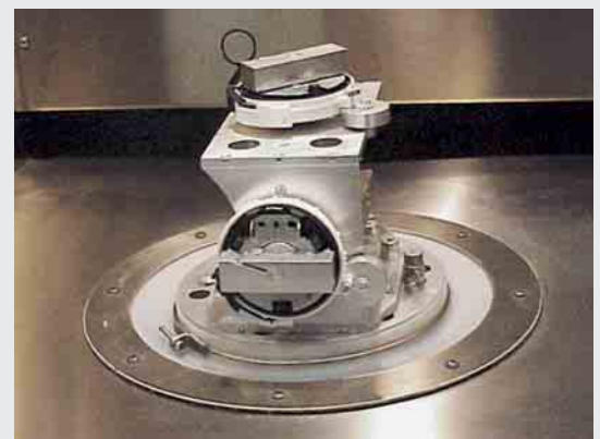
Diaphragms, inside and outside, to seal-off the vibration shaker with thermal barrier seated and interface to locate the test specimen
