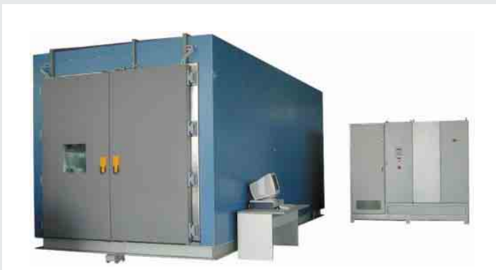
Walk- In climatic test chamber, 10 m 3
