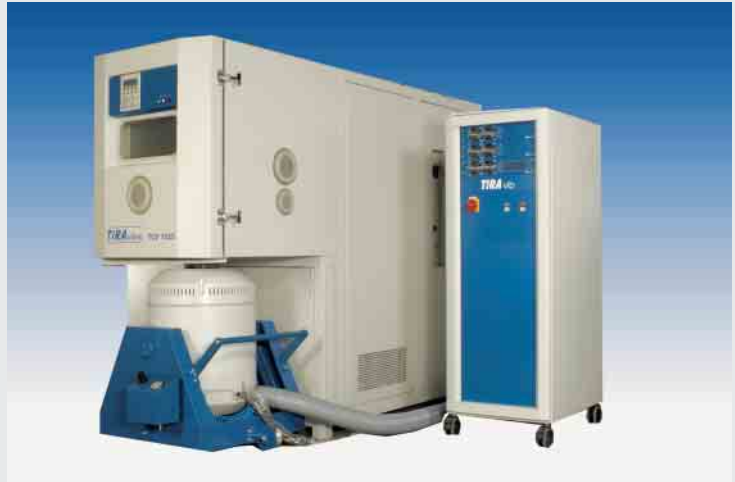
TIRA vibration test chamber system to match with vertical vibration shaker
