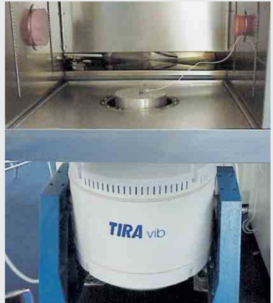
Internal view, Vibration test chamber with sliding floor and vertical shaker
